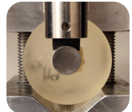
Shear bond test is conducted with 1 mm/min crosshead speed using an Instron model 5866.
